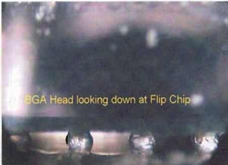
Figure 11: Standard BGA optics looks down at bottom fillet
